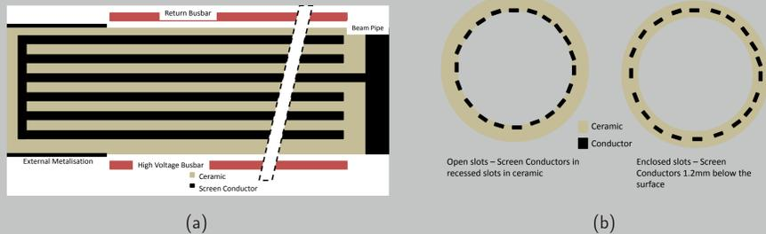
Figure 2: Cross sections of LHC-MKI beam screen with either 2(a) an alternative screen layout, in which most conductors are capacitively coupled at both ends, and 2(b) the beam screen in which the screen conductors are in enclosed slots rather than open slots.
