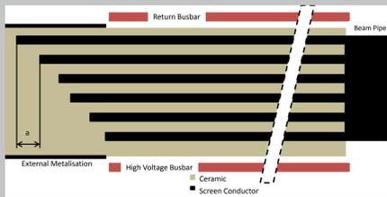
Figure 1: Illustrating the layout of the beam screen, with the screen conductors electrically connected to the beam pipe at one end of the screen, and capacitively coupled to the beam pipe at the other by an overlapping external metallisation.
