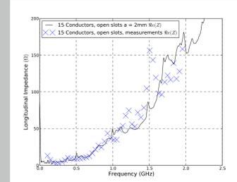
Figure 4: A comparison between the simulations and measurements of an LHC MKI with a beam screen with 15 screen conductors in open slots.
