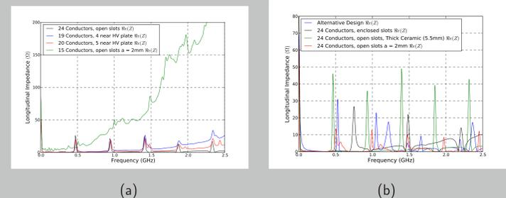
Figure 5: The longitudinal beam coupling impedance of 5 different numbers of screen conductors in the beam screen of the MKI and 5(b) different screen layouts for the MKI.
