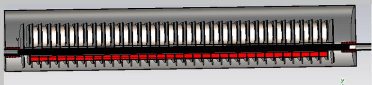
Figure 3: A cross section of the simulation model of the MKI. We see the transmission line kicker magnet structure with high voltage and ground plates, with capacitive plates in between. In red we see the ferrite yolk, and damping ferrites at the end of the structure to damp  $\lambda/4$  resonances of the screen conductors. The beam screen runs through the centre of the ferrite yoke.
