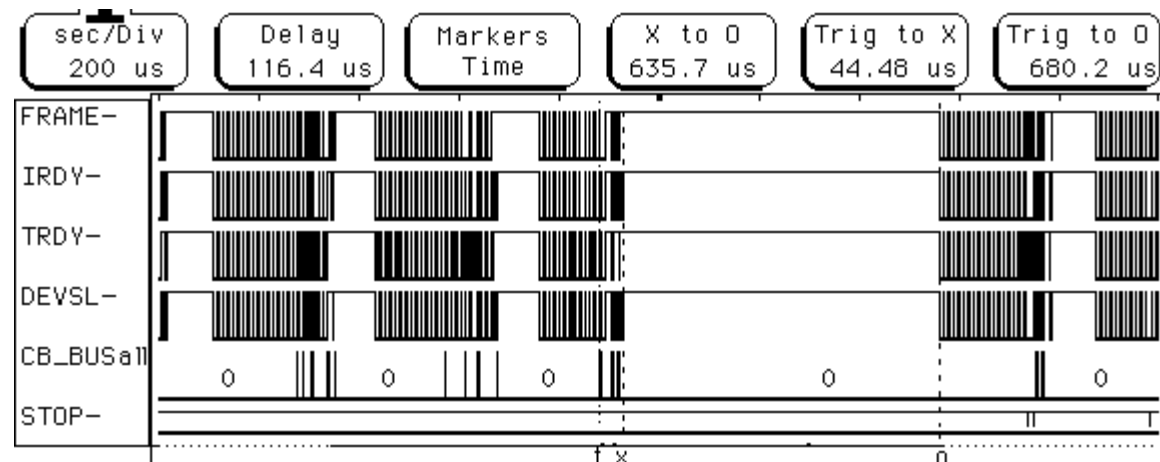
Figure 4.2 (d) PCI signals for the PC sending 1000 byte frames generated with a regular spacing of 20 ms. Note the CSR - data overlap during the first two sets of transfers and the long idle times.
