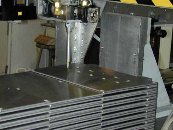
Gluing a stack of steel plates, leaving slots for tiles.
